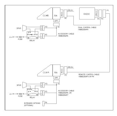
Figure 34 - ORION Dual Control Unit Remote Mount/Remote Mount Installation Configuration
